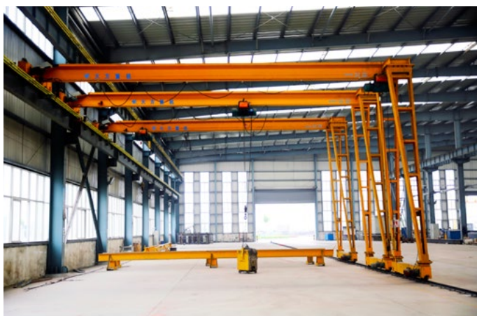
MHB 型电动葫芦半门式起重机 MHB type electric hoist semi gantry crane
