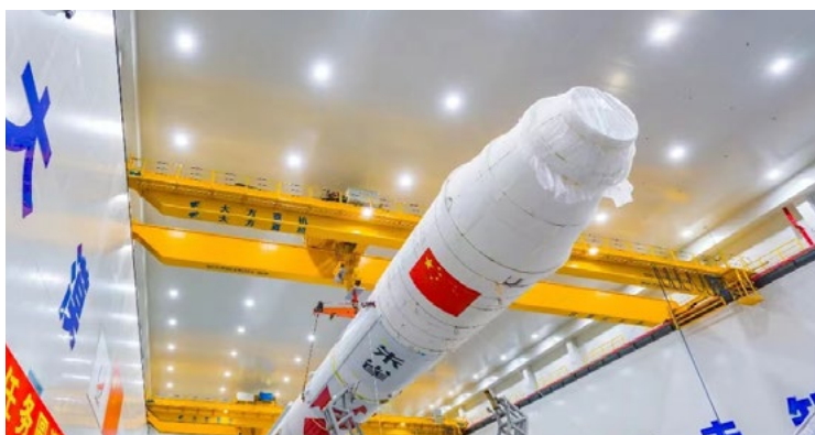
服务于全球首款液氧甲烷火箭朱雀二号 的大方造火箭发射专用起重机 The rocket launch crane serving the world's first liquid oxygen-methane rocket, Suzaku II
