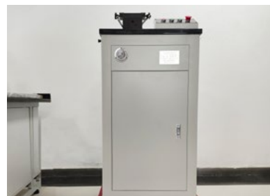
冲击试样缺口液压拉床 Hydraulic tensile machine for impact specimen gap
