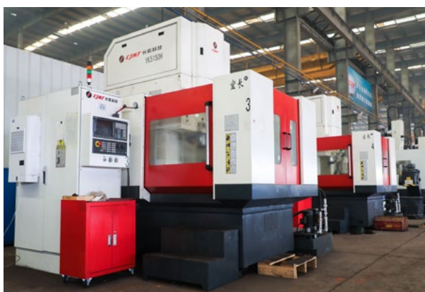
YT5180CNC 数控插齿机 YT5180CNC drilling machine
