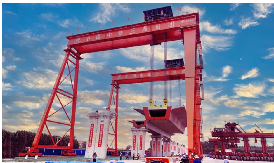
MG500+500t 提梁机 MG 500+500t girder lifting machine
